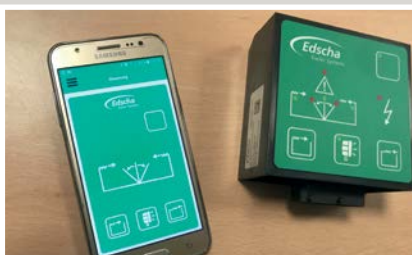
Operation with Android/iOS smartphone via our app and Bluetooth connection
