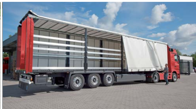
Opening the side curtains using the CS-Hybrid as an example
