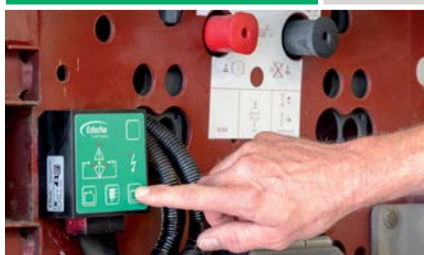
Operation directly on the control unit with inclinometer and overload protection
