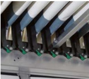
Dachaussteifung nach EN12642 XL Roof reinforcement in accordance with EN12642 XL
