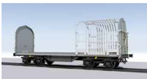
Railway SB · 示例: Shimmns 已打开的车顶
