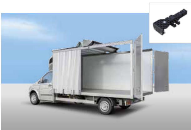
Compact 幕帘式车顶/全篷式滑动车顶
