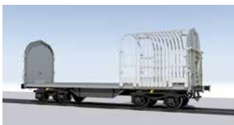
Railway SB · Example: Shimmns roof, opened
