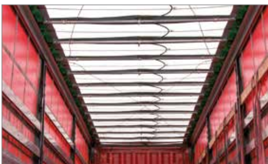
Komplette Integration in das Edscha Trailer Systems Schiebeverdeck Complete integration into the Edscha Trailer Systems sliding roof
